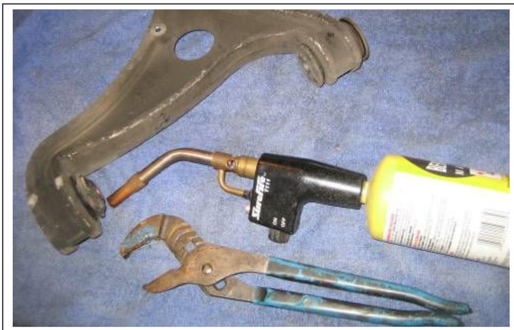
This helps de-bond the steel center bush. Extinguish the torch being careful to set it down in a safe place. Use Channel-locks to grab and rotate the steel bush back and forth. It will pull out of the rubber bushing with minimal effort. Do this for both front and rear steel top hat bushings. One at the front, two at the rear.
