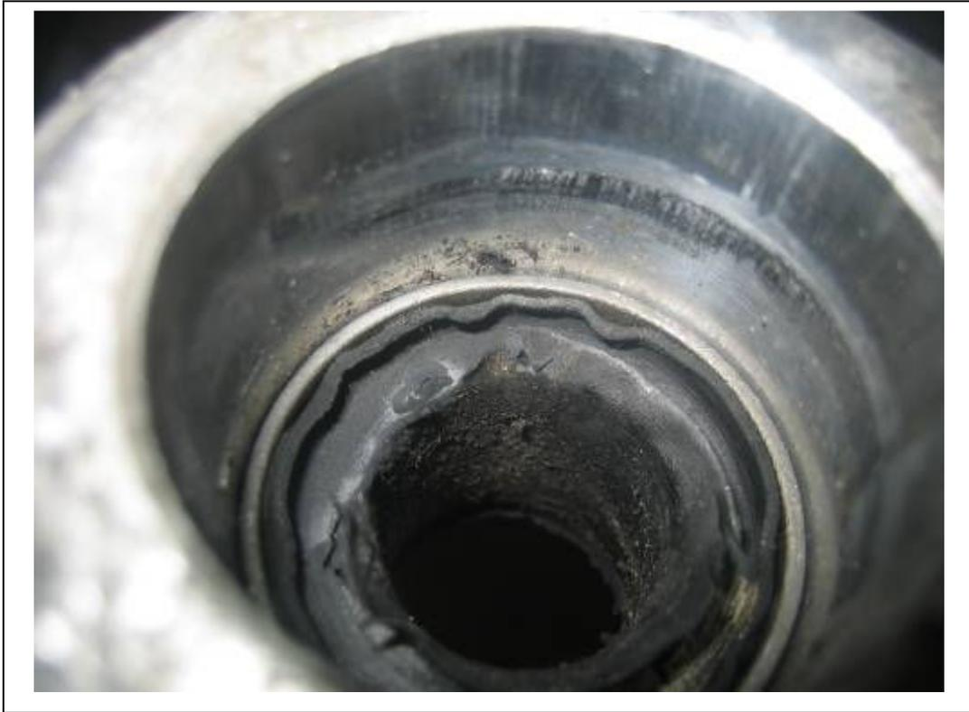
With sand paper or Scotchbrite, clean the bores of the control arms where the original rubber bushings were installed. It doesn't need to be shiny clean, just remove any highspots, dirt, rust etc. Remember the bushings do not rotate in the control arm.
