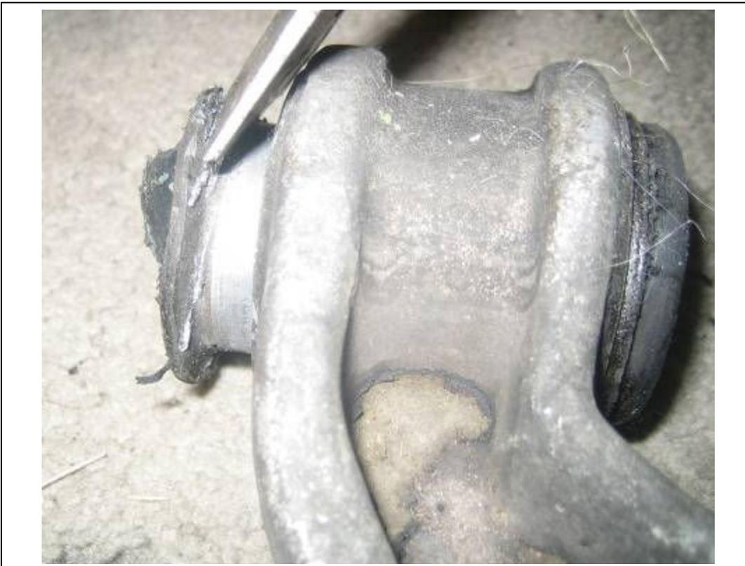
Once out, you will notice the other bushing can be easily punched out of the control arm from the inside.
