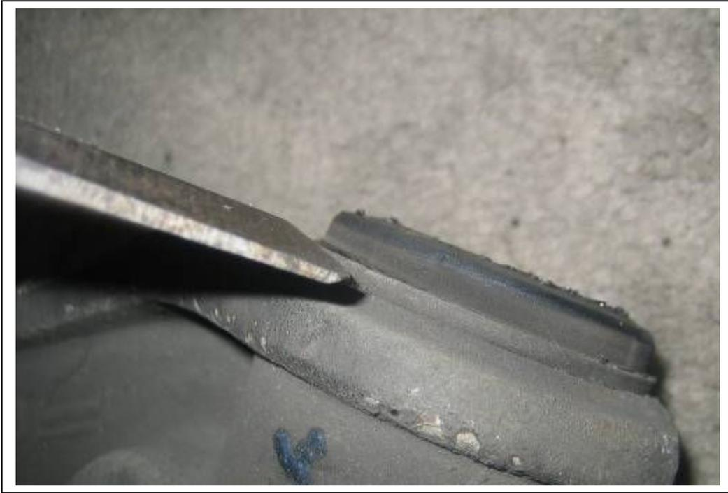
The steel flange of the rubber bushing will start to deform like this:
