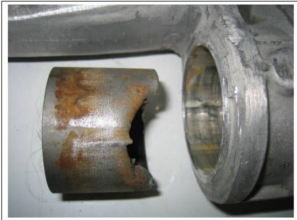
**Remove the Aft Bushings:** There are two bushings at the aft leg of the control arm. They are pressed into place to face each other. Use a large chisel to get under the steel lip of one of the outer bushing sleeves. Basically striking it at 90 degrees to the bushing centerline or axis. Work your way around the bushing sleeve flange.
