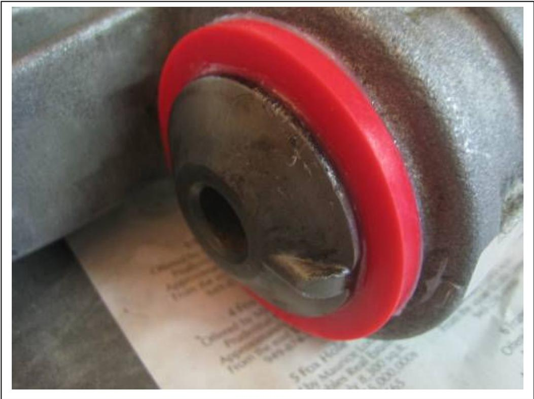
**Reinstall Control Arms:** You'll notice the forward steel pivot top hat bushing has a notch or locating feature that prevents the top hat bushing from turning while tightening its mounting bolt. The clocking or orientation of this top hat is important at the time the steel top hat is pressed into the urethane bushing. It is to be pointing towards the center of the car. See the above image for reference.
